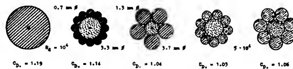
Figure 10. Fluid-dynamic drag coefficients of stranded wires, steel cables and ropes. Three items left by CAHI (12,a); two shapes right by AVA (12,c).
